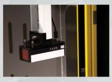
In addition to laser guarding, Sentinel enables connection of third party light curtains for the ultimate flexibility. For bending operations where light curtains are more suitable (eg. multi-height tooling), the operator can simply switch from laser protection to light curtain protection.
